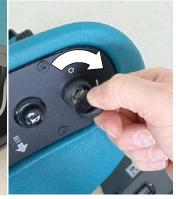
After the start position is set, manually turn the actuator tube until 3.25 in (8.26 cm) of thread is exposed as shown.
